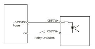
Sensor And Switch Connection
