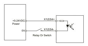
Sensor And Switch Connection
