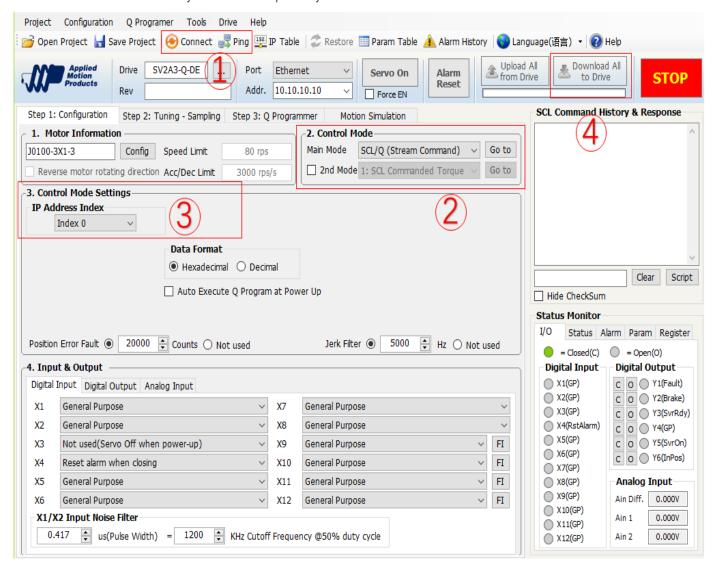
For SV200 series drives, there are 16 index values for 16 different IP addresses. Default address are as shown in table below:
