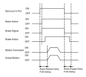
Brake engage/disengage delay time can be set via SVX ServoSUITE®, or on the drive directly via P function: P-69 (BD) or P-70 (BE).
