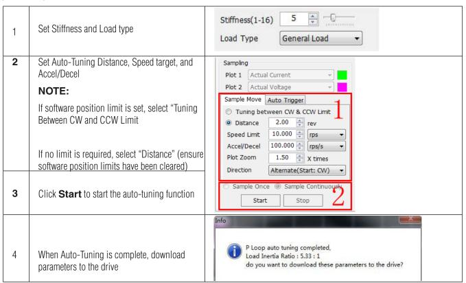
NOTE: During the tuning process, motor or load vibrations may occur. This is normal and the system will correct itself.
