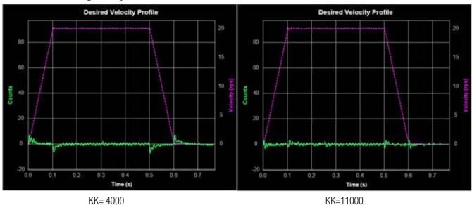
When the feedforward (KK) gain is too large, however, the opposite effect can be seen. This will also decrease system dynamic performance by increasing position error and system settling time, as shown below.
