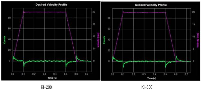
As seen below, if KI is too large, the whole servo system will vibrate and make noise. This, in turn, will increase the position error and may greatly extend settling time due to system oscillations around the target position.
