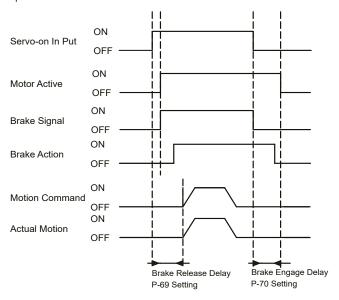
The Brake Output (BO) setting can be configured with the SVX Servo Suite software or with parameter P-67(BO), as shown in the table below. Brake disengage delay and engage delay times can be configured via SVX ServoSUITE®, or by changing parameters P-69 (BD) and P-70 (BE) directly from the drive.
