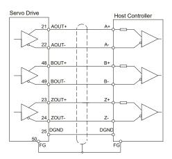
NOTE: Please make sure the host controller and the servo drive are connected to a common ground.
