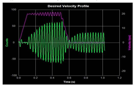
As seen below show, the position error is reduced as KV increases.
