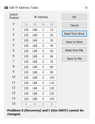
**Read from Drive:** IP the IP table from the connected drive **Save to Drive:** Save current IP table values to the drive.
