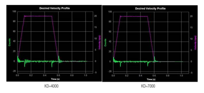
When KD is too large, however, the system will become highly sensitive to the commanded changes in motion, which can potentially cause unexpected system vibrations and noise as shown below.
