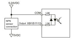
Sensor And Switch Connection
