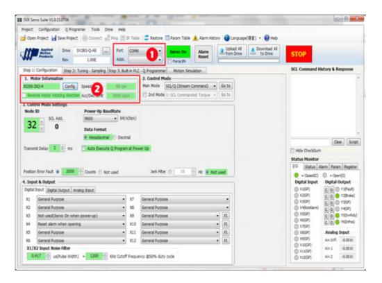
Step 3: click on motor "Config" button and select motor model from drop-down list.
