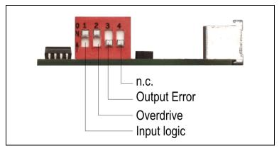
Fig. 17: DIP switches on the board
