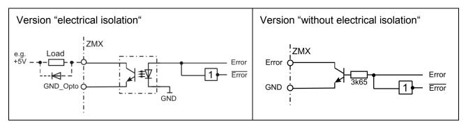
Abb. 1: Output wiring diagram
