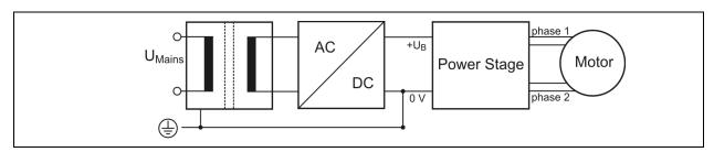
Fig. 6: PELV – Grounding: 0 V
