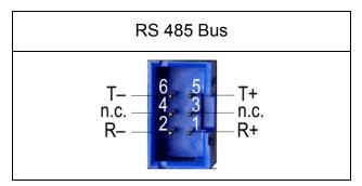
Fig. 12: ServiceBus connector type Tyco Electronics 2-1761605-1/609-0607
