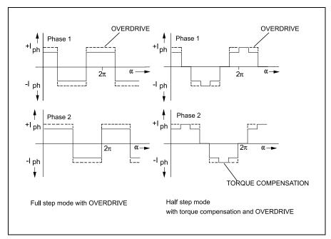
With increasing step frequency the stepper motor phase current decreases, caused by the counter electromotive force of the motor. The amplitude of the current shape is smaller and the motor looses torque.
