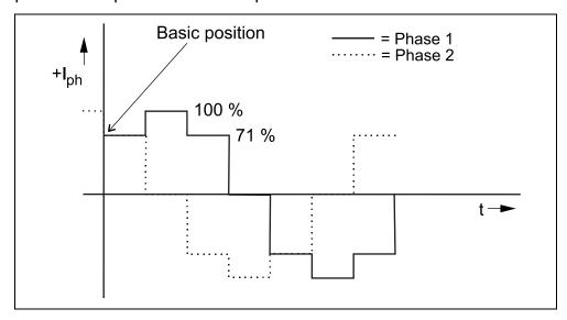
Fig. 22: Motor phases in basic position (half step)
