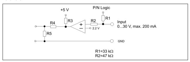
Fig. 21: Input circuit "without electrical isolation"
