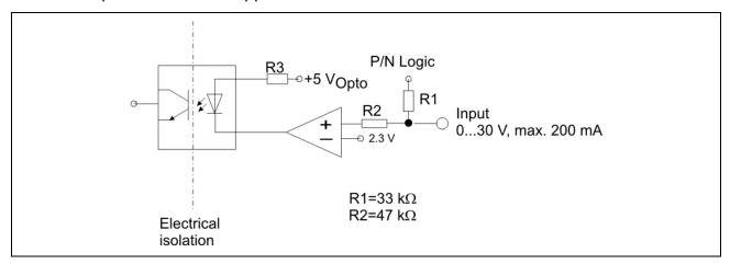
Fig. 20: Input circuit "electrical isolation"
