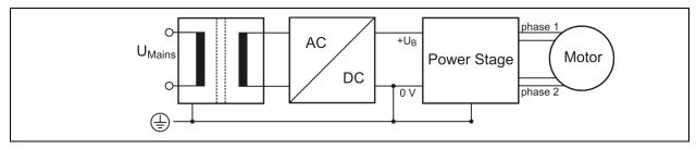
Fig. 5: PELV – Grounding: 0 V and Power Stage
