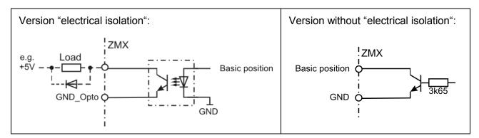
Fig. 23: Output wiring "BASIC POSITION" without electrical isolation
