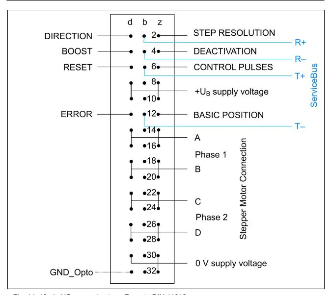
Fig. 14: 48 pin VG connector, type F acc.to DIN 41612
