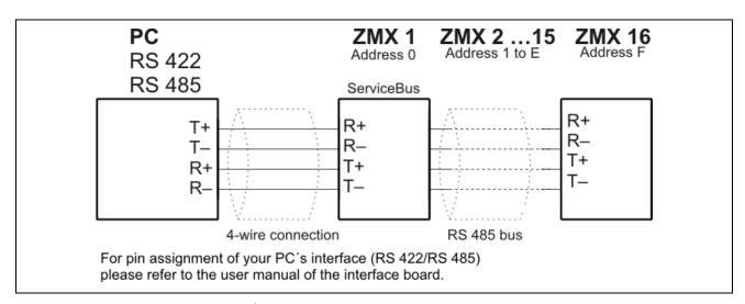
Fig. 19: Connection PC -> ZMX<sup>+</sup> with RS 422/RS 485 interface
