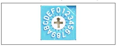
Fig. 15: 16-step rotary switch: Setting 0...F
