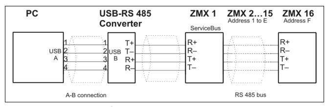
Fig. 18: Connection PC -> ZMX<sup>+</sup> via USB/RS 485 converter
