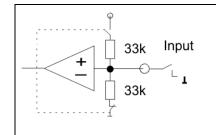
2. Connecting ground and high impedance
