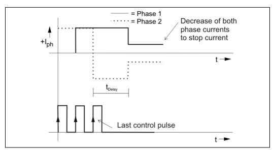
Fig. 25: Decrease to stop current after the last control pulse (full step)
