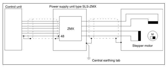
Fig. 7: Motor cable shielding
