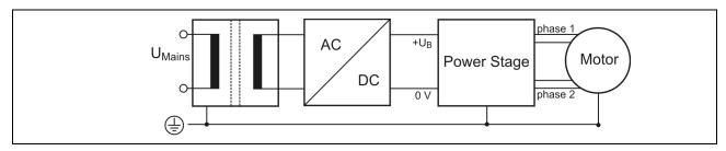
Fig. 3: PELV – Grounding: Power Stage and Motor. The secondary winding of the transformer (SELV supply) must not be grounded because the equipment is grounded.
