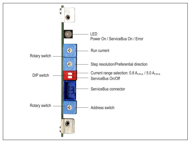
Fig. 1: Control components
