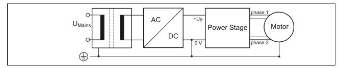
Fig. 4: PELV – Grounding: 0 V and Motor
