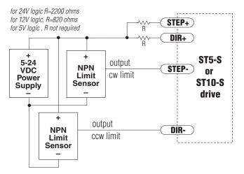
If the sensor output goes low at the limit, select the option "closed" (DL1). If the output is open, or high voltage, choose "open" (DL2).
