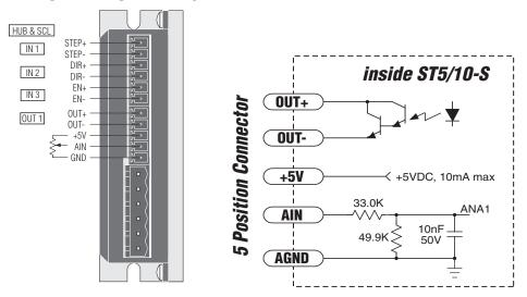
The ST5-S and ST10-S drives include one digital output that can be used in one of five ways:
