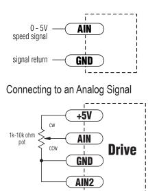
Connecting the Analog Signal to a Potentiometer or Joystick
