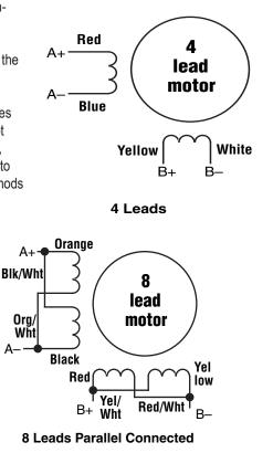
Eight lead motors can also be connected in two ways: series and parallel. As with six lead motors, series operation gives you less torgue at high speeds, but may result in lower motor losses and less heating. In series operation, the motor should be operated at 30% less than the unipolar rated current. The motors recommended in this manual should be connected in parallel. The wiring diagrams for eight lead motors are shown on the following page.
