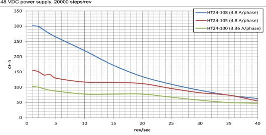
HT24 48 VDC power supply, 20000 steps/rev
