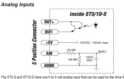
The ST5-S and ST10-S have one 0 to 5 volt analog input that can be used by the drive for controlling the motor speed in velocity mode. This input can also be used to read a voltage using the SCL "IA" or "RA" commands.
