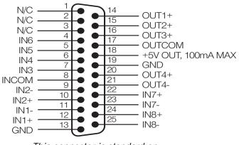
This connector is standard on -Q and -IP models.
