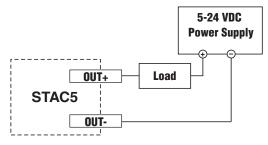
Sinking Output Using Y1, Y2 or OUT4
