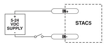
**Connecting a Mechanical Switch to Low Speed Differential Inputs**
