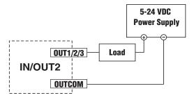
Sinking Output Using OUT1, OUT2 or OUT3
