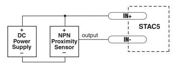
**Connecting an NPN Proximilty Sensor to Low Speed Differential Inputs**
