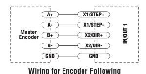
(Encoder power can be supplied from the +5V OUT terminal on IN/OUT 1 if the encoder requires no more than 100mA)
