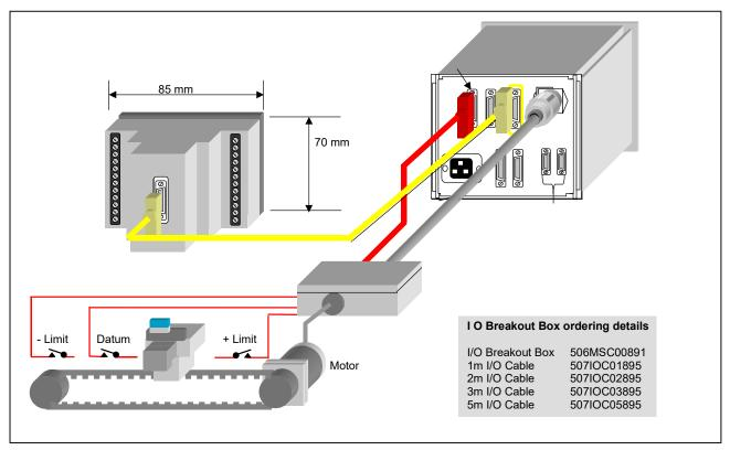
Fig. 9.1 I/O Breakout Box and I/O Cable
