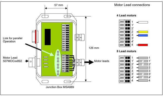
Fig. 4.4 Parallel Motor Coil Connections
