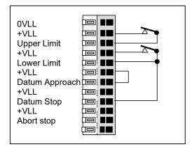
Fig. 4.6 Limit/Datum Connections
