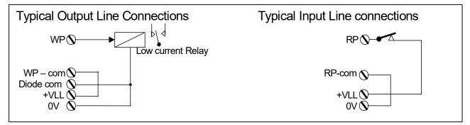
Fig. 9.3 Typical Connections to the I/O Breakout Box
