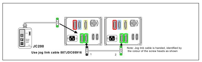
Fig. 7.2 Dual axis installations
