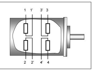
Fig. 4.1 Eight lead 23 & 34 frame size motors
