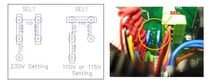
Fig. 5.1 Mains Voltage Selector
