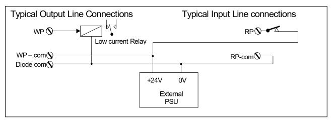
Fig. 9.4 Typical I/O Connections using an External Supply
