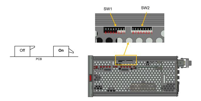
Fig 6.1 MSE570M Switch layout
