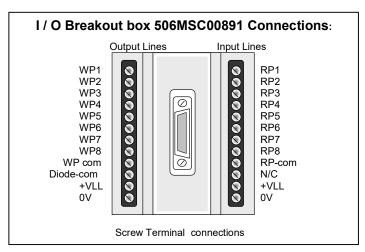
Fig. 9.2 I/O Breakout Box Connections
