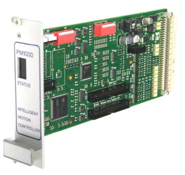
The MSE1000 is a microprocessor-based unit for controlling servo or stepper motors. When fitted with a front panel (as shown above) the controller is referred to as a PM1000. This panel is not used in the Sim-Step. The controller has a wide range of functions available and these are described in detail in the PM1000 manual included with this documentation.
