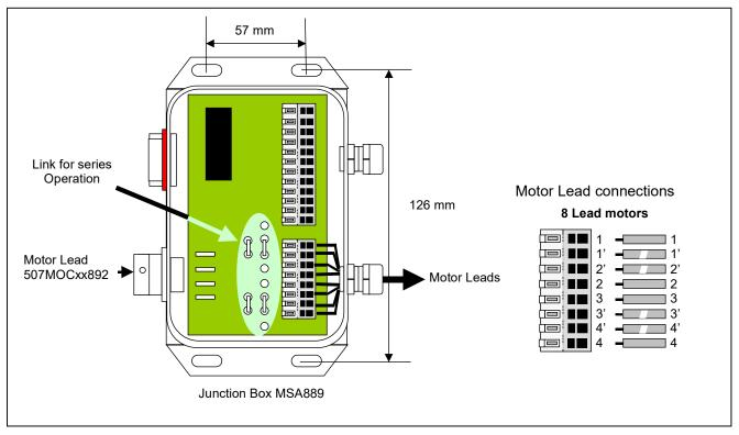
Fig. 4.5 Series Motor Coil Connections
